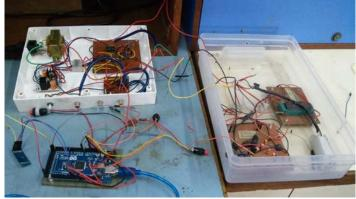
Out of the three parameters anyone of the parameters could be selected first. Here the Pulse Rate was selected first. The button connected to pin 6 was pressed, connection was made and the Arduino started reading the values. The app was launched, all the details were filled and then the Pulse Rate
